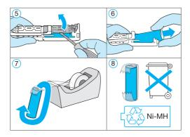
Open the handle as shown, remove the battery and dispose of it according to local environmental regulations.
