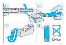
Open the handle as shown, remove the battery and dispose of it according to local environmental regulations.
